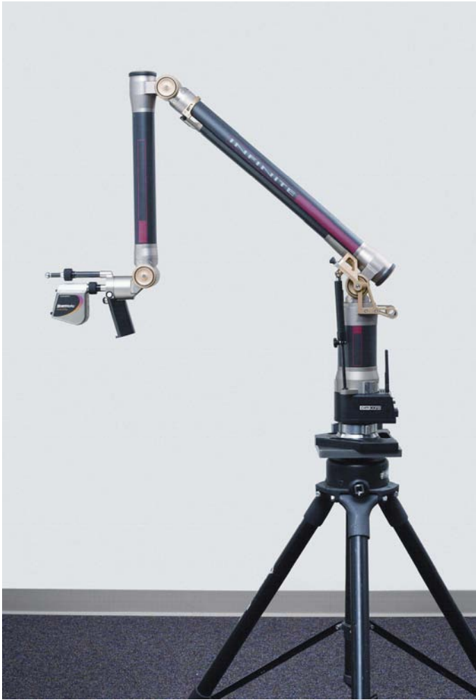
Figure 5. Laser Scanning System with Portable CMM Arm (photo courtesy Perceptron Inc.)
