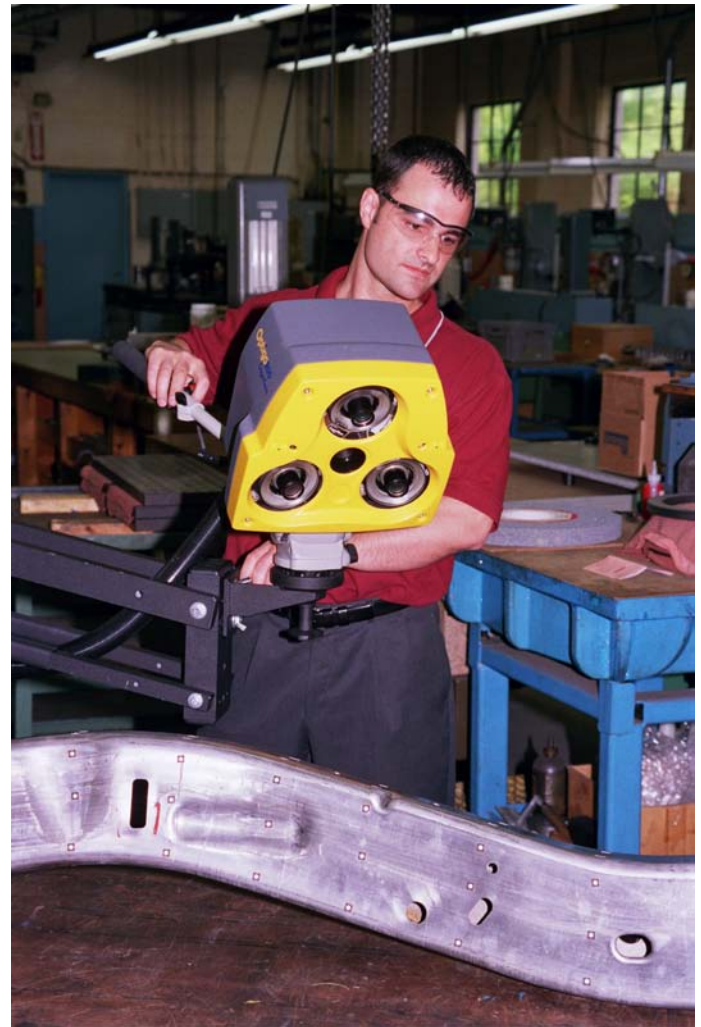
Figure 6. White Light Photogrammetry System (photo courtesy CogniTens Inc.)
